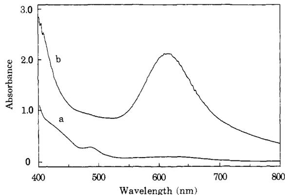
Figure 1. Electronic spectra at  $-40\text{ }^{\circ}\text{C}$  in  $\text{CH}_3\text{CN}$  (0.1-cm path length) of (a) **1** (6.1 mM) and (b) **1** (6.1 mM) + 1.5 equiv of  $\text{H}_2\text{O}_2$ .
